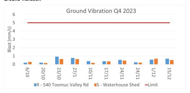
Figure 6 - Blasting; Ground Vibration Results Q4 2023 (Limit is 5mm/s for 95% of blasts in a 12 month period)
