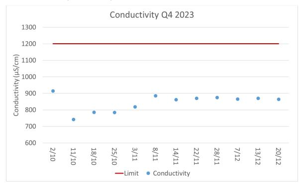
Figure 10 - Discharge Water Conductivity results Q4 2023
