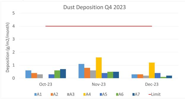
Figure 4 - Dust Deposition Q4 2023. (Limit 4.0g/m2/mth)
