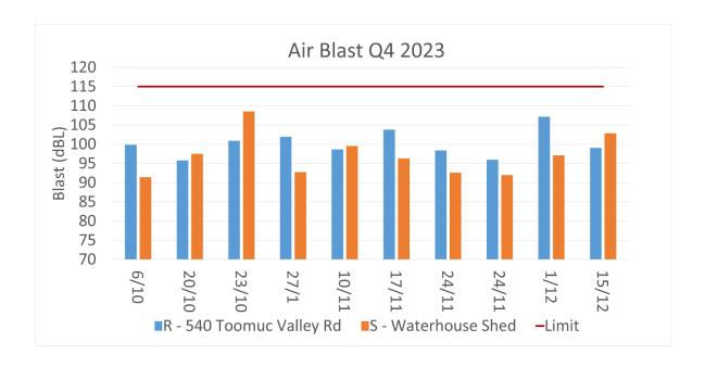
Figure 7 - Blasting; Air Blast Results Q4 2023 (Limit is 115 dBL for 95% of blasts in a 12 month period)
