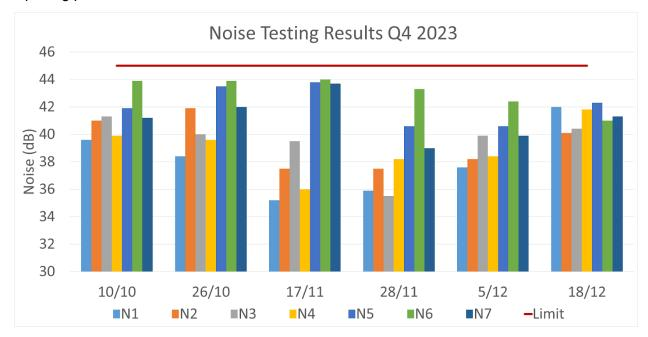
Figure 5 - Noise Testing Results Q4 2023. (Limit is 45dB under normal operating conditions)
