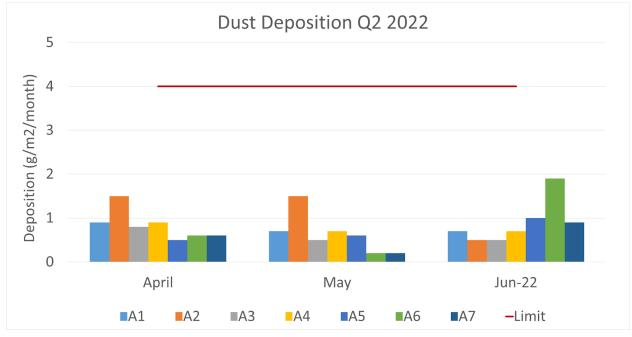
Figure 3 - Dust Deposition Q2 2022. (Limit 4.0g/m2/mth)
