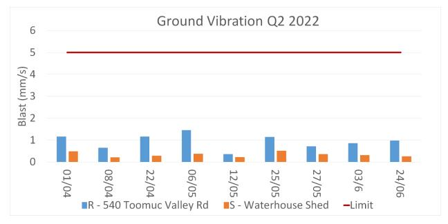
Figure 5 - Blasting; Ground Vibration Results Q2 2022 (Limit is 5mm/s for 95% of blasts in a 12 month period)
