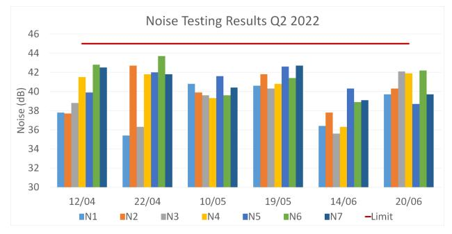
Figure 4 - Noise Testing Results Q2 2022. (Limit is 45dB under normal operating conditions)
