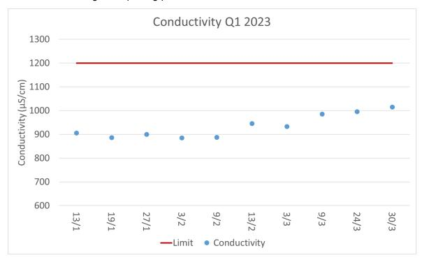
Figure 10 - Discharge Water Conductivity results Q1 2023
