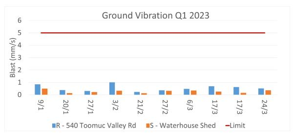
Figure 6 - Blasting; Ground Vibration Results Q1 2023 (Limit is 5mm/s for 95% of blasts in a 12 month period)
