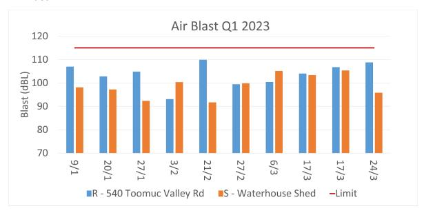
Figure 7 - Blasting; Air Blast Results Q1 2023 (Limit is 115 dBL for 95% of blasts in a 12 month period)
