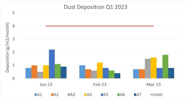
Figure 4 - Dust Deposition Q1 2023. (Limit 4.0g/m2/mth)
