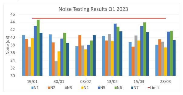
Figure 5 - Noise Testing Results Q1 2023. (Limit is 45dB under normal operating conditions)
