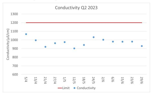
Figure 10 - Discharge Water Conductivity results Q2 2023
