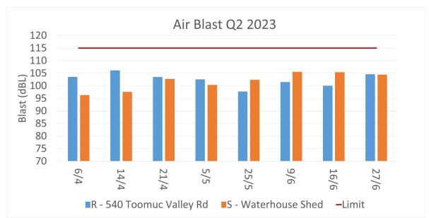
Figure 7 - Blasting; Air Blast Results Q2 2023 (Limit is 115 dBL for 95% of blasts in a 12 month period)
