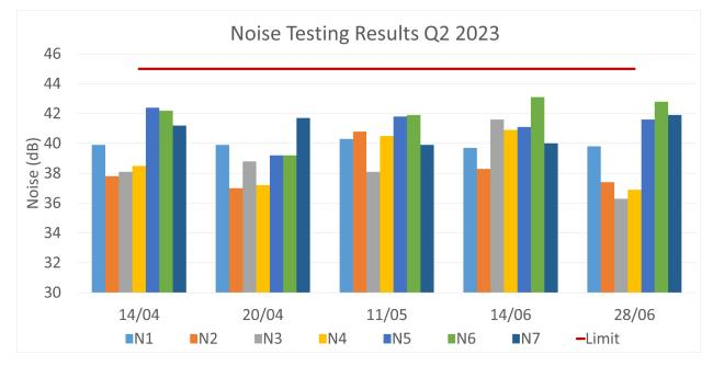
Figure 5 - Noise Testing Results Q2 2023. (Limit is 45dB under normal operating conditions)
