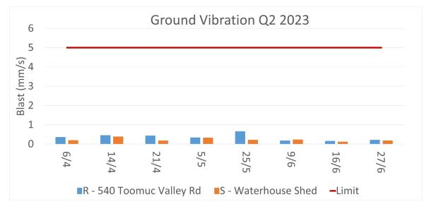
Figure 6 - Blasting; Ground Vibration Results Q2 2023 (Limit is 5mm/s for 95% of blasts in a 12 month period)
